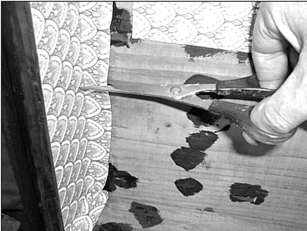
*Cutting the top on a curved top trunk. Make about six to eight cuts evenly spaced along the curve to keep the liner from bunching.*
